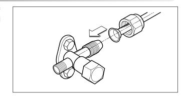
Finally, tighten the flare nut with torque wrench until the wrench clicks.
